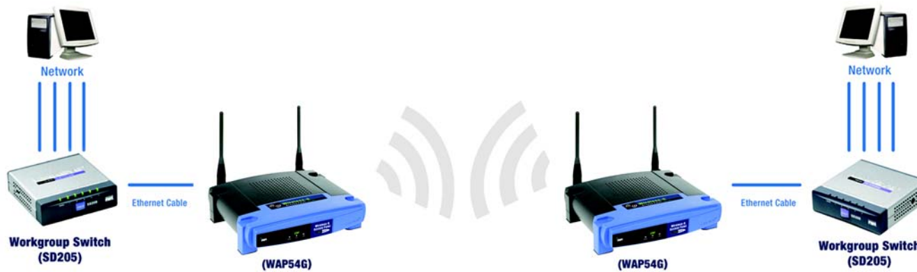
Figure 7-7: Wireless Bridge Diagram
