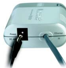
Figure 3-7: Connect Power to the Injector
