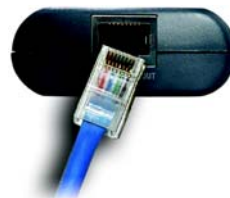
Figure 3-6: Connect the Ethernet Cable to the Injector
