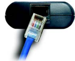
Figure 3-2: Connect the Ethernet Cable to the Injector
