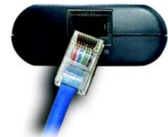
Figure 3-3: Connect the Ethernet Cable to the Splitter
