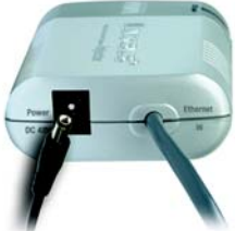
Figure 3-5: Connect Power to the Injector
